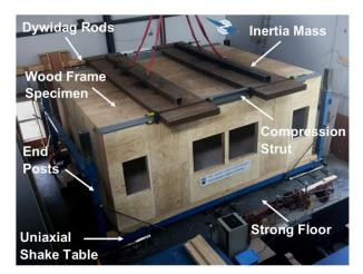
Figure 4.6. Full-Scale Test Setup
