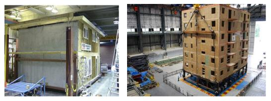
Figure 4.1. Photograph of Type-2 house and NEESWood building at full-scale shake table
